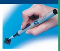
Our PEN-VAC® line offers a replacement for SMD tweezers. The soft suction cup material will not scratch your parts or damage delicate leads. This is an excellent tool for pick-and-place of many standard and odd size SMT components.
